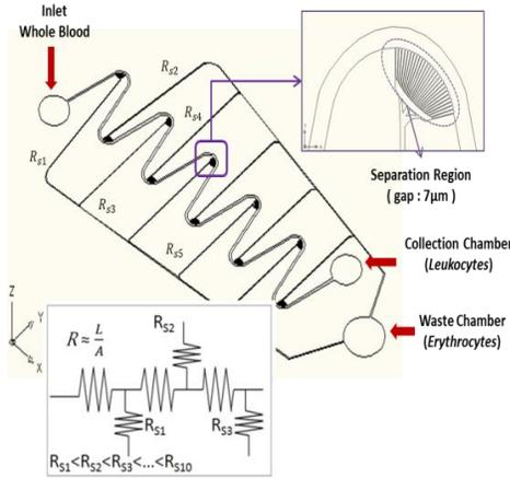
Fig. 2: Microfluidic channel geometry. 200µm(W) x 70µm (H) with symmetrically curve channels along main channel.
