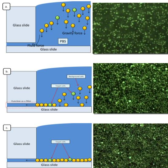
Fig. 4. Schematic cross-sectional view of the cells aligning process
