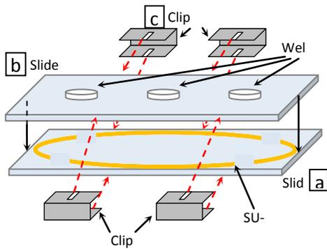
Fig. 5 System assembly schematic diagram
