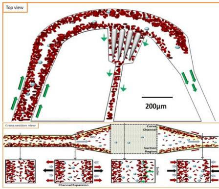
Fig. 1: Schematic of cells migration in confined main channel and absorption along inner-wall of curve channel. Particles in flow experience drag and lift forces yield the particles to equilibrium position as shown at channel cross section.
