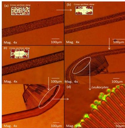
Fig. 3: (a) Whole blood cells at initial flow in channel. (b) Human blood cells with 20X buffer dilution begin to migrate at inner-wall by increasing the injection flow rate (1mL/min.). (c) Cells crowded by increasing the blood cells concentration with 5X of buffer dilution. (d) Leukocytes in the curve channel rejected at (~7µm) entrance of separation region.
