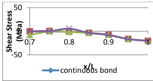
Figure 9: Shearing stress distribution of FEM results for bi-layered assembly with continuous and partial bond
