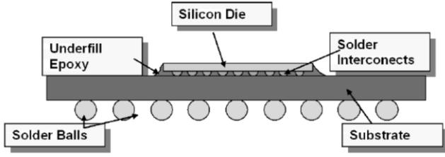
Figure 6(a): Flip Chip Ball Grid Array [19]
