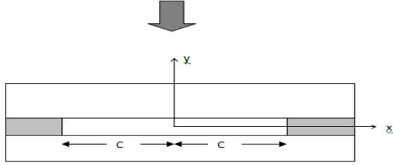
Figure 6(b): simplified schematic diagram of FCBGA assembly with partial bond [16]
