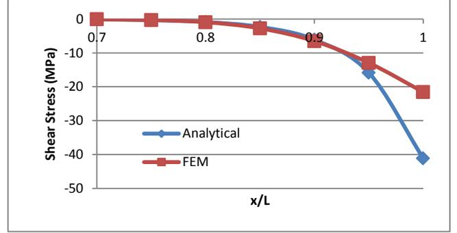
Figure 2: Comparison of shearing stress between analytical and FEM solution
