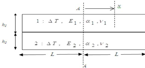
Fig. 1(a): Geometric and material parameters of the bi-layered model
