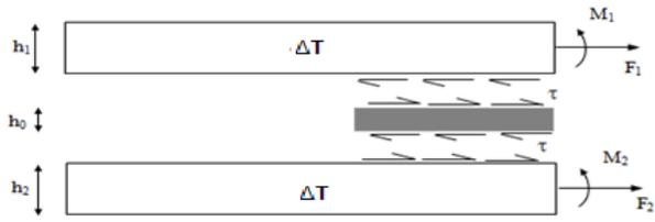
Figure 7: Free body diagram of bi-layered assembly with partial bond
