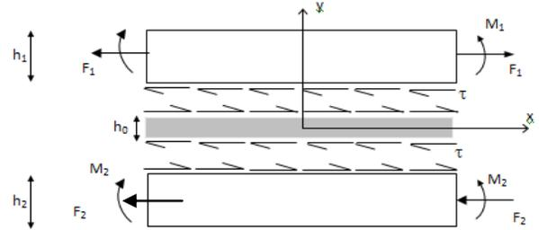
Figure 3: Free body diagram of bi-layered assembly with continuous bond
