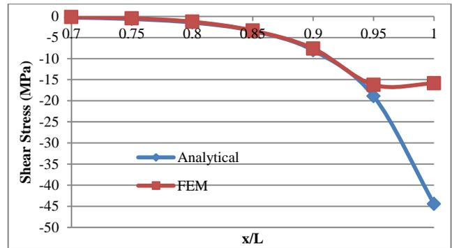
Figure 5: Comparison of shear stress between analytical and FEM solution for bi-layered assembly with continuous bond
