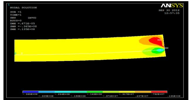
Figure 4: Shear stress distribution in FEM model for bi-layered assembly with continuous bond
