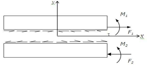
Fig 1(b): Free-body diagram of the bi-layered model
