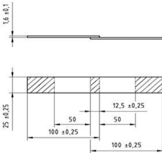
Fig. 1 Configuration and dimensions of lap shear bonded specimens
