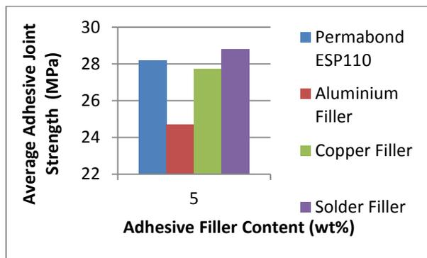
Fig. 3 Effect of powder additions on the lap shear strength of the adhesive joints
