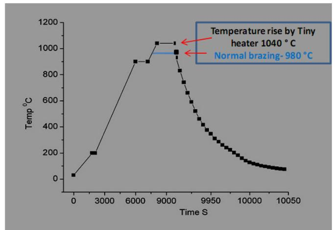
Fig 2. Brazing cycle (Brazing temperature: 1050° C, Quenching pressure: 1300 m.bar)
