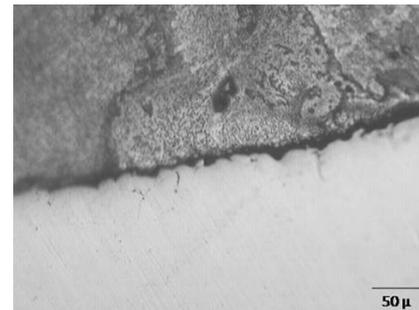
Fig 5. Microstructure of joint for various brazing temperatures: a) 980°C b) 980°C with tiny heater on PHSS part, c) 1040° C.
