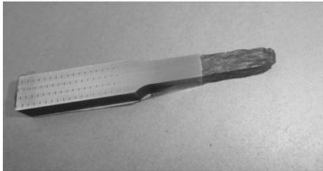
Fig. 4. Tensile test sample after testing.
