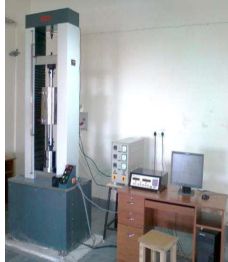
Figure 2: Computer controlled UTM of 100kN capacity with resistance heating three zone furnace
