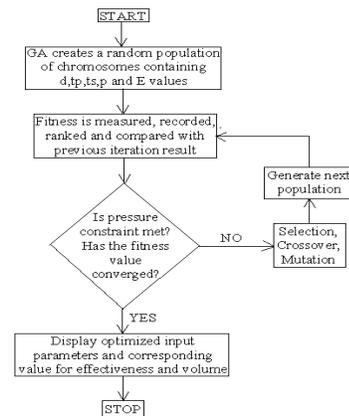
Figure 4. Flow chart of a simple coded GA
