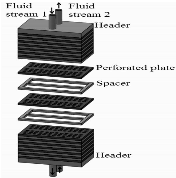
Figure 1. Perforated plate heat exchanger
