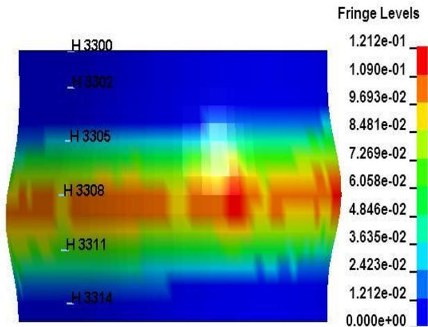
Fig. 3 Distribution of magnetic field on tube
