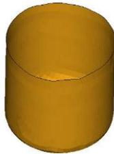
Figure 9. Cup drawn with modified blank-2
