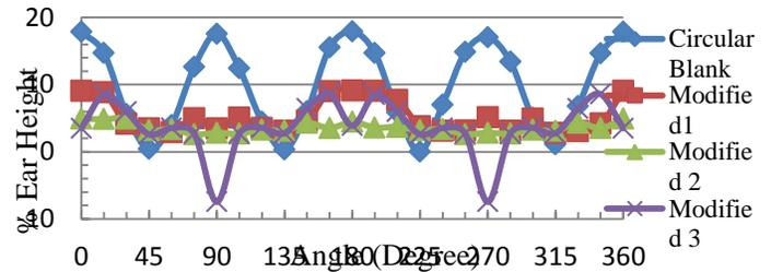
Figure 11. Comparison of earing profile of different modified initial blanks in cylindrical deep drawing in terms of % ear height
