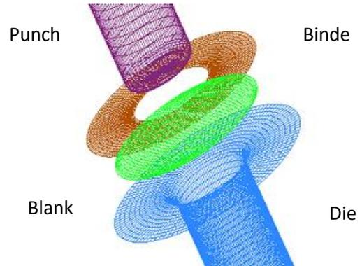
Figure 3. Exploded view of FE model of cylindrical deep drawing
