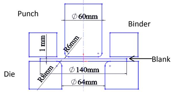
Figure 2. Schematic view of toolings used in deep drawing process.
