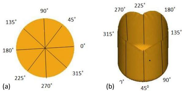
Figure 4. Cup height measurements at different places on (a) initial blank and (b) deformed cup
