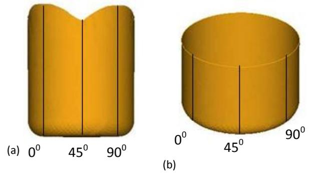
Figure 6. Earing profile predicted incorporating (a) Hill's and (b) Von Mises yield criteria
