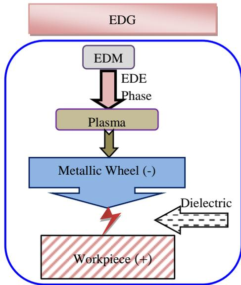
Fig 1 Elements of electric discharge grinding (EDG)
