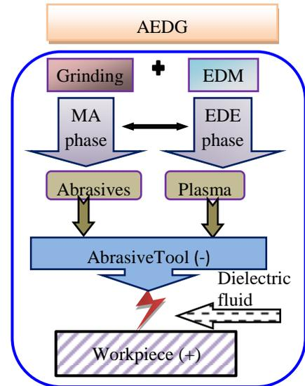
Fig 2 Elements of abrasive electro discharge grinding (AEDG) process [1]
