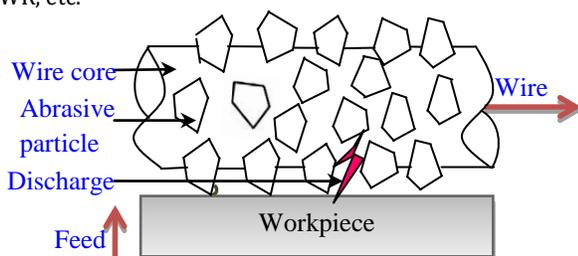
Fig 5 Schematic diagram of abrasive WEDM process
