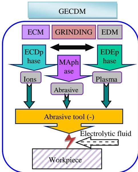
Fig 7 Elements of grinding assisted electro-chemical discharge machining (GECDM)
