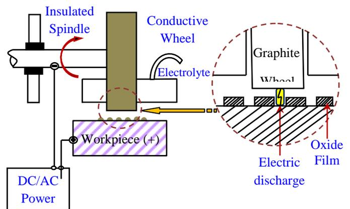
Fig 3 Schematic of electro chemical diamond grinding (ECDG) process
