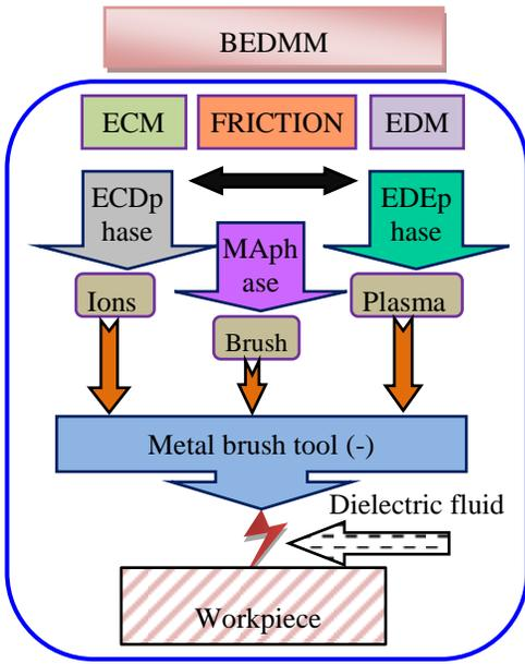
Fig 6 Elements of brush erosion-dissolution mechanical machining (BEDMM)
