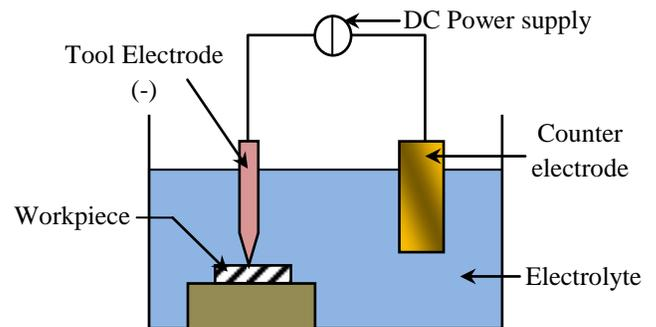
Fig 4 Schematic of electro chemical discharge machining (ECDM) process
