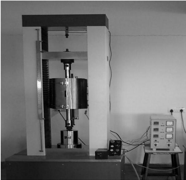
Figure 1: Computer controlled UTM of 100kN capacity with Resistance heating three zone Split Furnace
