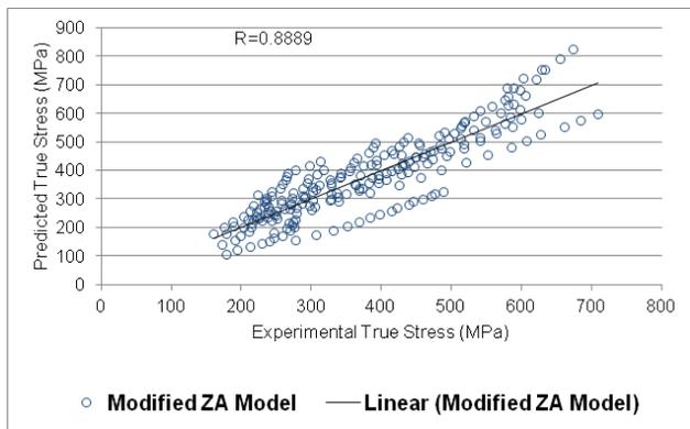
Figure 4: Plot of predicted vs experimental stress for Modified - ZA Model.
