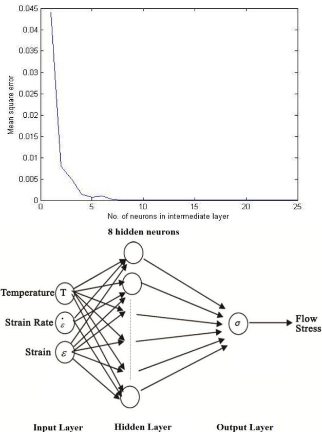
Figure 3: (a) Plot of mean square error (MSE) vs. no. of intermediate neurons in the ANN architecture, (b) ANN architecture (3-8-1)
