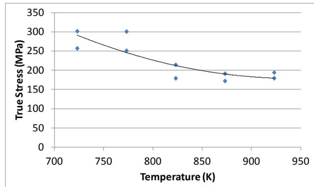
Figure 2: Plot of true stress and temperature at 0.0001 s<sup>-1</sup> strain rate for modified ZA model.
