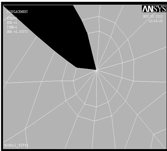
Figure 8 - Deformed shape in the vicinity of the crack tip
