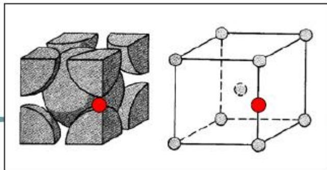
Figure:  $\alpha$ -Iron BCC Lattice with Hydrogen Interstitial
