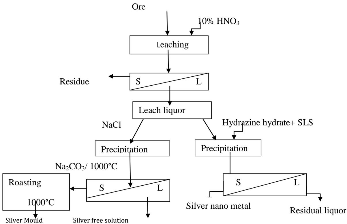
Fig. 6 Flow sheet for silver metal production
