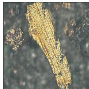
Figure-3.3: Severe Sliding
