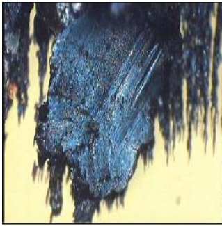
Figure-3.5: Gear Wear
