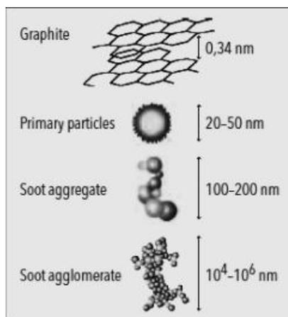
Figure 3: Size comparisons of individual particles of tire running surface
