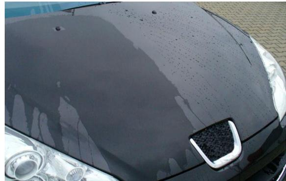
Figure 2: The difference with and without hydrophobic nano coating.
