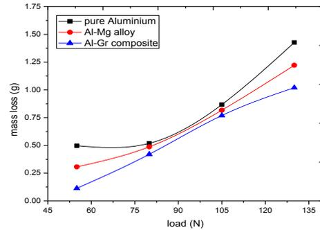
Fig. 3: Mass loss vs. load in dry sand abrasion test
