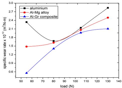
Fig. 4: Specific wear rate vs. load in dry sand abrasion test
