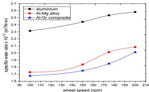
Fig. 2: Specific wear rate vs. wheel speed in dry sand abrasion test
