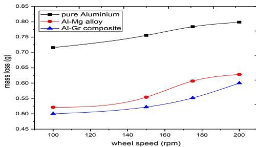
Fig. 1: Mass loss vs. wheel speed in dry sand abrasion test
