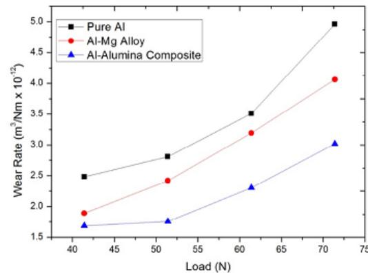
Fig 5 : wear rate Vs load
