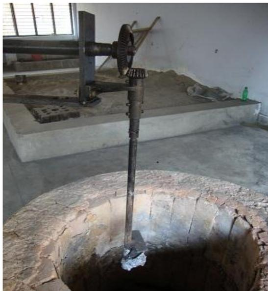
Fig. 1 Stir casting setup
