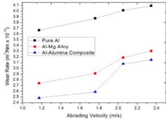
Fig 4: Wear rate Vs Abrading Velocity
