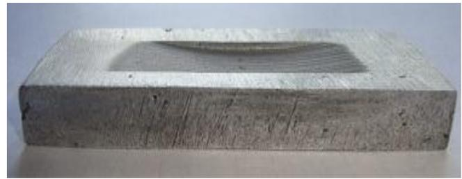
Fig 3 Tested Specimen of Casted Composite
