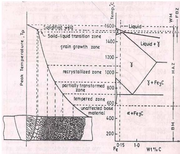
Fig: Different welding zone
