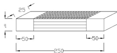
Where, t= thickness of the specimen
