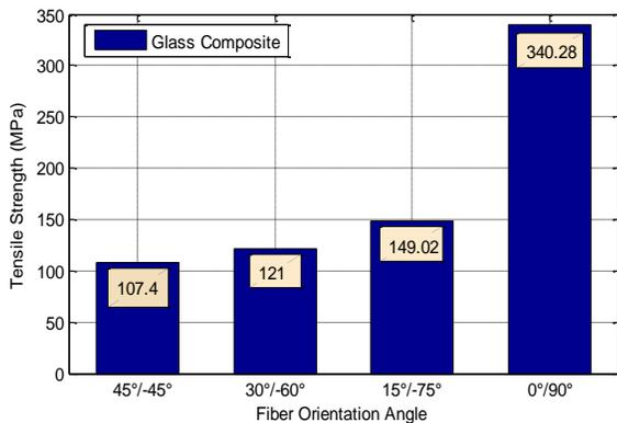
Fig. 10: Effect of Fiber Orientation on Tensile Strength of Glass Composites.
