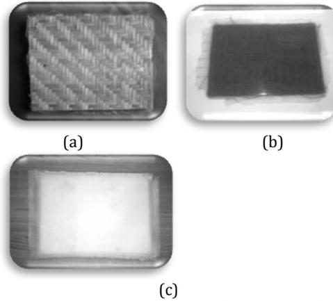
Fig. 2(a-c): Casted bamboo, jute, and glass laminates.
