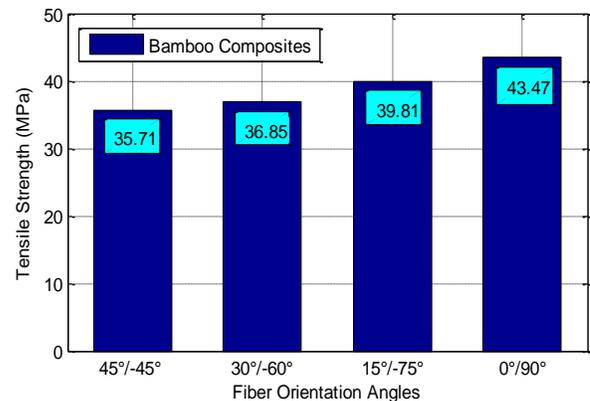
Fig. 8: Effect of Fiber Orientation on Tensile Strength of Bamboo Composites.
