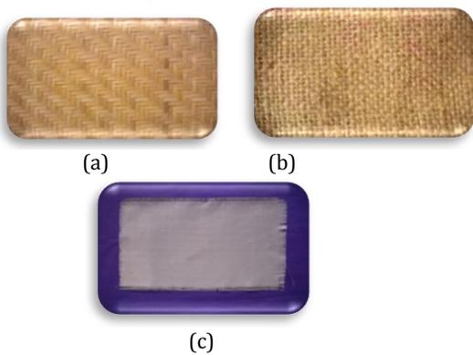
Fig. 1(a), 1(b) and 1(c) shows bamboo, jute, and glass fiber in mat form.
