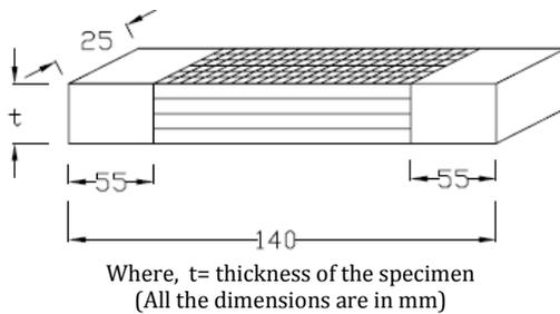
Fig. 6: Geometry of specimen for compression test
