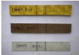
Fig.5: Composite specimen for compressive test
