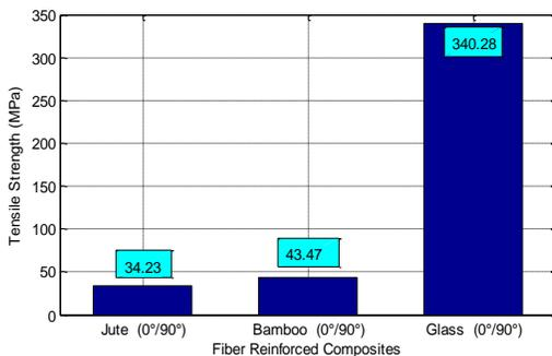
Fig. 11: Comparison of Tensile Strength of Jute, Bamboo, and Glass Composites.
