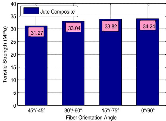
Fig. 9: Effect of Fiber Orientation on Tensile Strength of Jute Composites.
