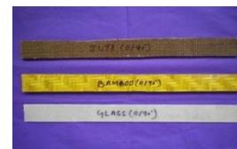
Fig.3: Composite specimen for tensile test
