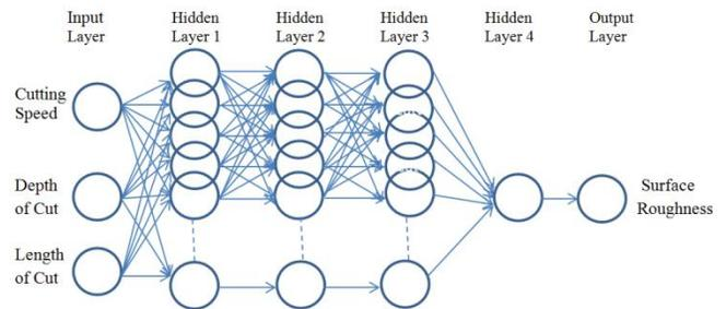
Figure 1: Configuration Of The Neural Network
