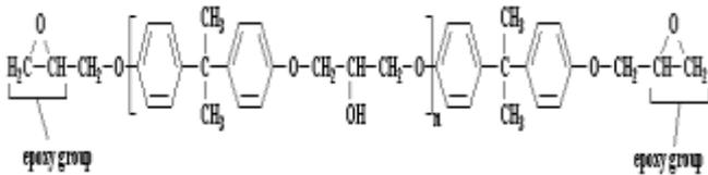
Epoxies generally out-perform most other resin types in terms of mechanical properties and resistance to environmental degradation, which leads to their almost exclusive use in aircraft components.
