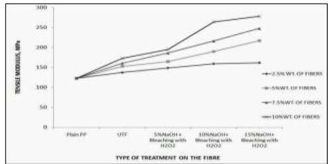
Figure 3.2: effect of chemical treatment and % wt. of fiber on tensile modulus of continuous long jute fiber reinforced PP composites
