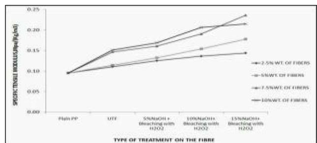
Figure 3.5: effect of chemical treatment and % wt. of fiber on specific tensile modulus of continuous long jute fiber reinforced PP composites
