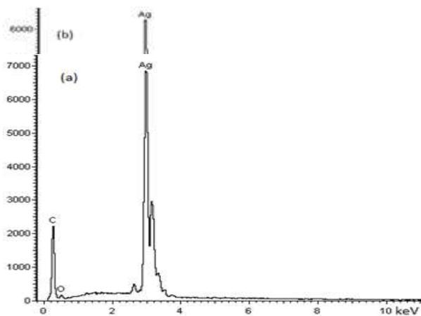
Figure 2. EDAX spectra of silver nanoparticles prepared at (a) pH 6 (b) pH 10.
