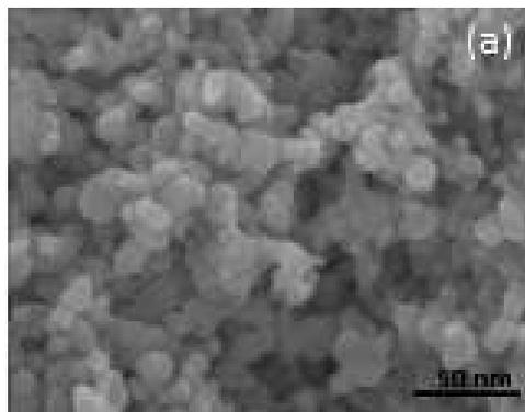
Figure 3. FESEM images of silver nanoparticles at a) pH 8 (b) pH 10
