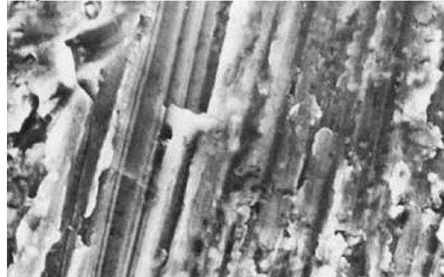
Fig. 1 Scanning of electron micrograph of LM13/8%MgO
