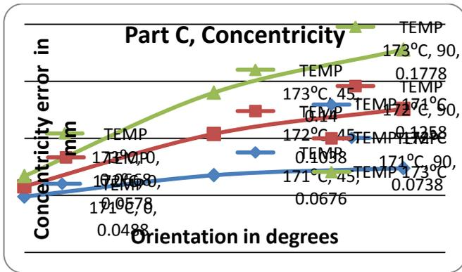
Fig.7 Effect of orientation angle and sintering temperature on concentricity error
