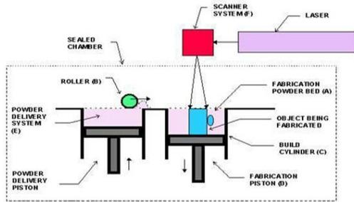
Fig.1 Schematic diagram of Selective laser sintering process
