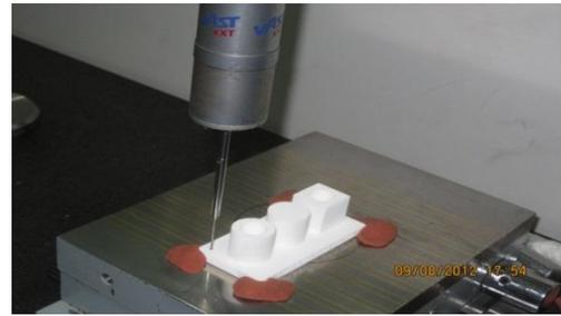
Fig.4 Inspection of the benchmark part on CMM
