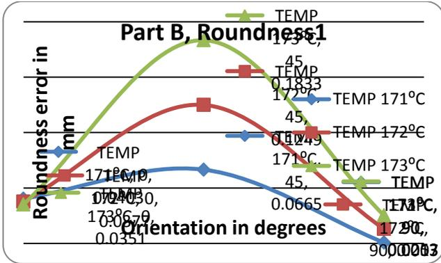
Fig. 6 Effect of orientation angle and sintering temperature on roundness error
