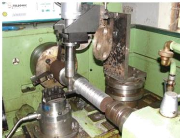
Figure4. Work piece preparation in UAT using lathe (HMT Model NH 26).
