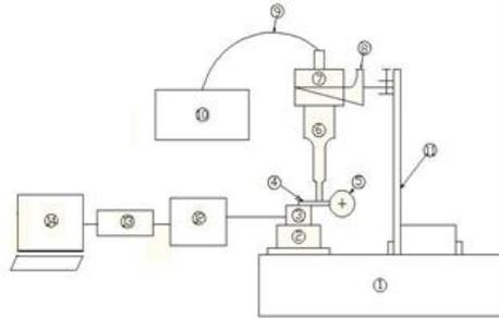
Figure2. 2-D Schematic diagram of ultrasonic assisted turning System.
