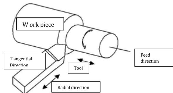
Figure1. Principal vibration directions during ultrasonically assisted turning[5].
