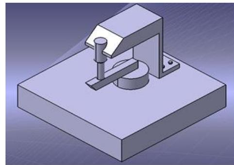
Figure3. 3-D view of experimental set up (Cutting tool treated as cantilever beam).
