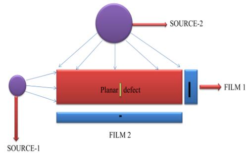
Fig-5 side view of weld sample for multi-shot examination in radiography
