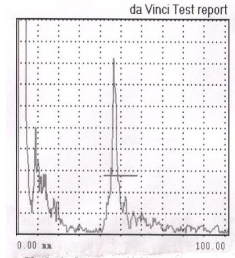
Fig-4: Graphical representation of defect of da vinci alpha Ultrasonic flaw detector
