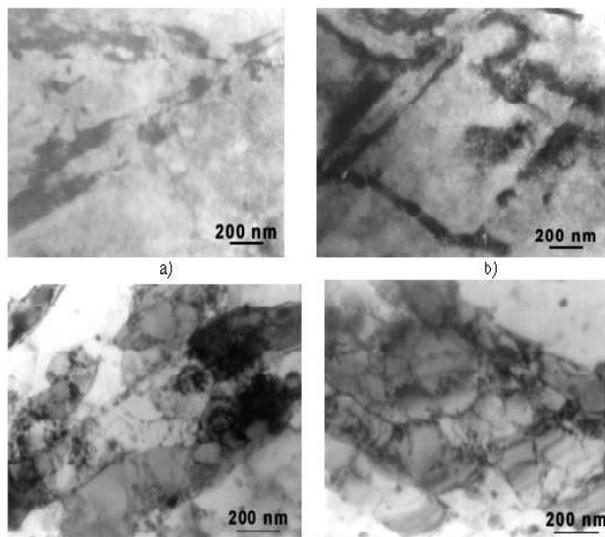
Fig 7. Substructure of Aluminum alloy 6082 after extrusion: a) after the 1st pass, b) after the 2nd pass, c) after the 3rd pass, d) after the 4th pass
