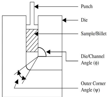
Fig 1. Schematic Illustration of ECAP
