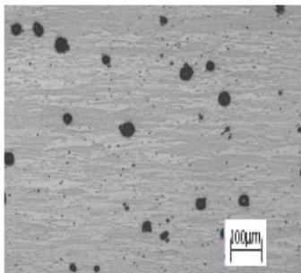
Fig 6. Structure of Initial Sample (before ECAP)
