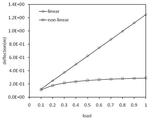
Fig. 11 Variation of deflection with respect to load
