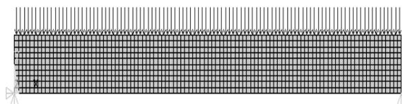
Fig. 1 2-D FE model showing meshing, boundary conditions, and loading (s=10, a=0.2)
