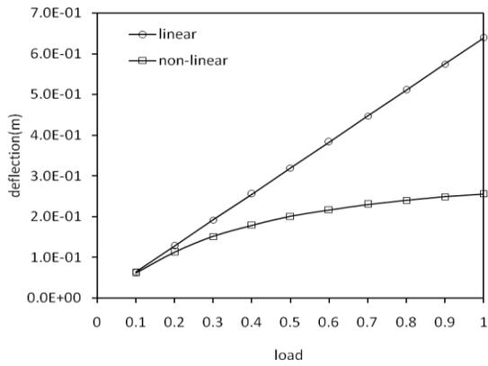
Fig. 9 Variation of deflection with respect to load
