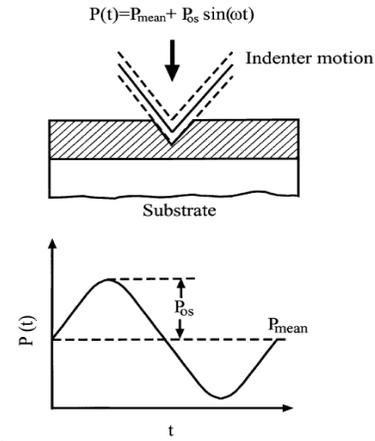
Fig 2: Schematics of a fatigue test made on a thin-film/ substrate system by the Nanoindentation technique.
