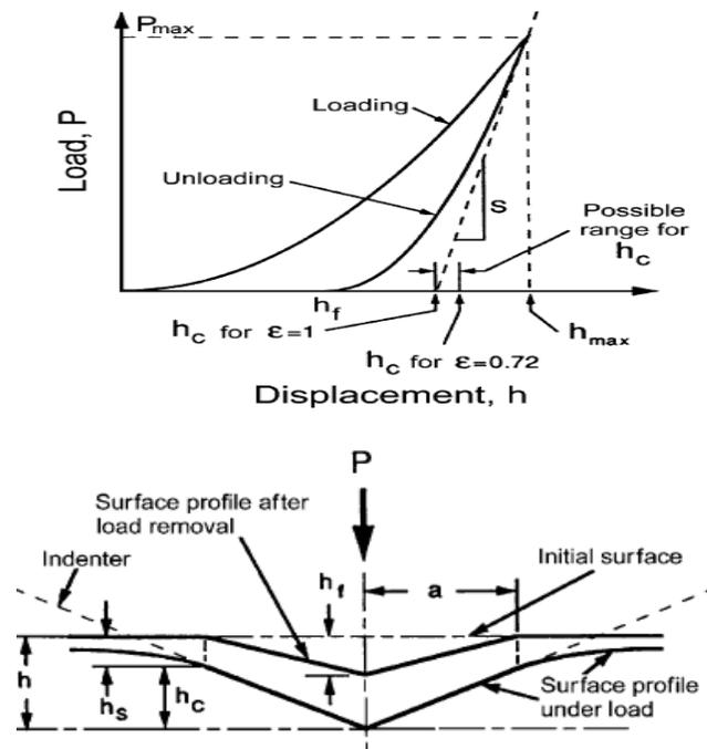
Fig 1. Typical Load displacement curve and the deformation pattern in sample
