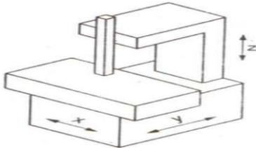
Column type structure is very rigid and accurate. The Z-axis is connected to the arm and the table moves independently in the X and Y-axis. The constructional difference in column type with the cantilever type is with x and y-axis movements.
