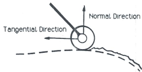
Fig- Chamfering pass.
