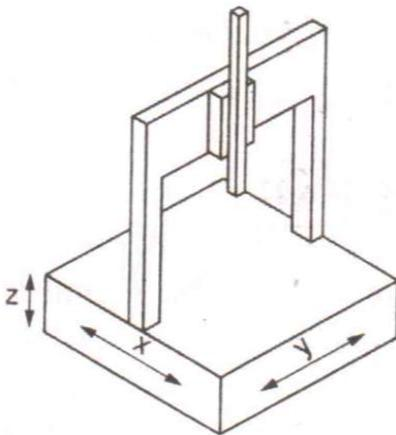
The bridge type structure is similar to the cantilever type because of the Y-axis support. The bridge construction adds rigidity to the machine, but both ends of the Y-axis must track at the same rate. Loading the machine part can be difficult at times because there are two legs that touch the base.
