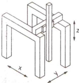
For the gantry type structure, support of the workpiece is independent of the X and Y axes, which are overhead and supported by four vertical columns rising from the floor. One can walk along a workpiece with the tool, which is helpful for very large workpieces.
