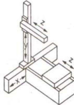
In the horizontal type arrangement, the tool is carried along the Y-axis moving arm. The Y-axis arm moves up and down on a column for Z-axis travel, and the column can move along the edge of the work table in the X direction. It has a very large, unobstructed work area, which makes it ideal for very large parts.
