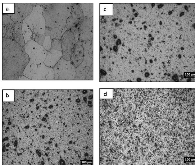
Figure 1: Optical images of: (a) Pure Titanium (b) Ti+B4C (165µm) (c) Ti+B4C (49µm) (d) Ti+B4C (8µm)
