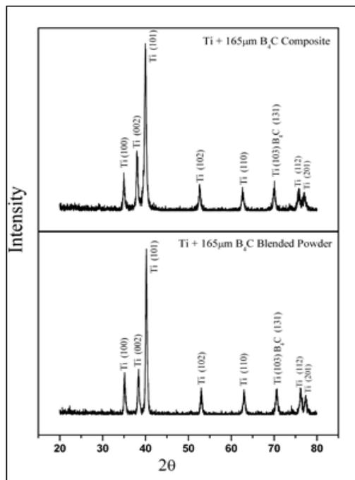
Figure 2: X-ray diffraction patterns of TMC with 165 µm B4C before VHP (bottom) and after VHP (top)
