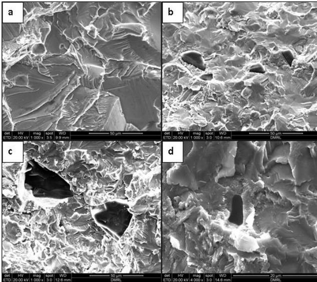
Figure 3: SEM fractographs of (a) Pure titanium (b) Ti+B4C (165µm) (c) Ti+B4C (49µm) (d) Ti+B4C (8µm)
