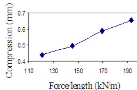
Figure 5: Aluminium circular wire-seal compression against force per unit length.
