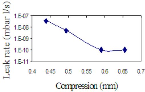
Figure 6: Aluminium circular wire-seal leak rate against compression.
