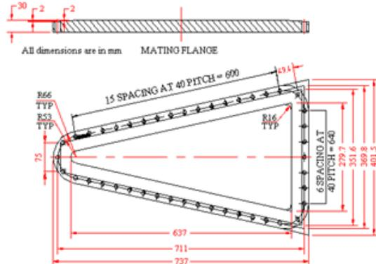
Figure 1: Triangular port blanking flange.
