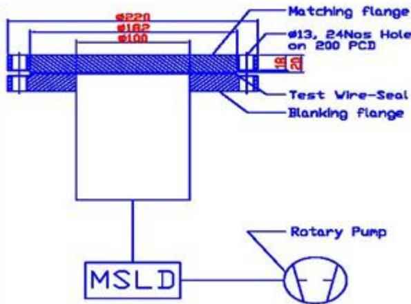
Figure 3: Schematic of the experimental set-up with circular flange.
