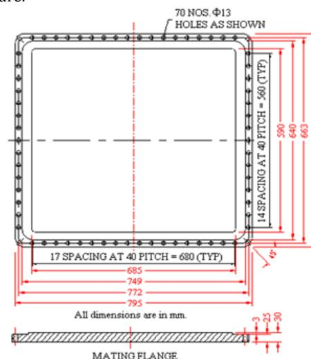
Figure 2: Rectangular port blanking flange.
