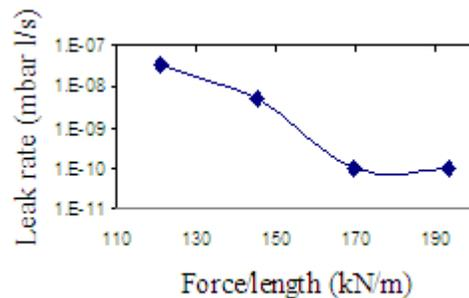
Figure 4: Aluminium circular wire-seal leak rate against force per unit length.
