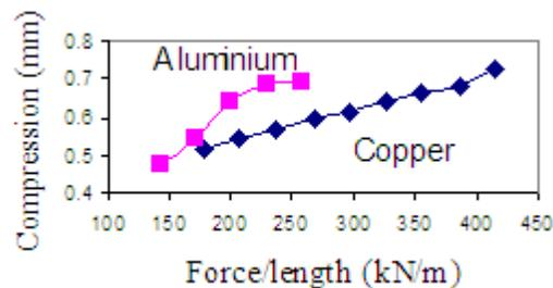
Figure 8: Triangular wire-seal average compression against force per unit length.
