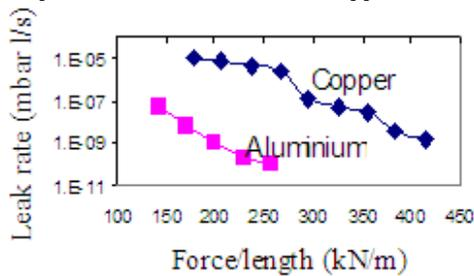
Figure 7: Triangular wire-seal average leak rate against force per unit length.
