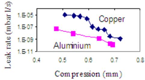
Figure 9: Triangular wire-seal average leak rate against average compression.
