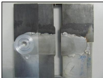
Fig. 4 Tensile sample taken out from the sample by EDM cutting
