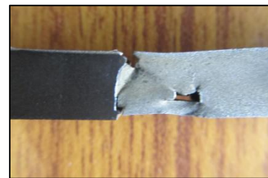
Fig. 6 Formation of void in the advancing side
