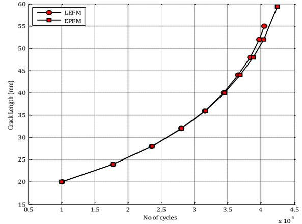
Figure 3. Fatigue life variation with crack length for a center crack plate.
