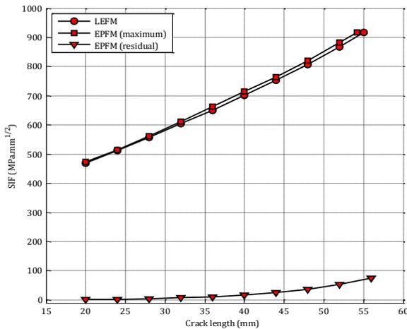
Figure 2. SIF variation with crack length for a center crack plate.
