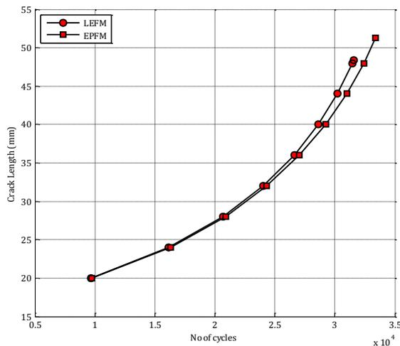
Figure 6. Fatigue life variation with crack length for a center crack plate in the presence of multiple holes, inclusions and minor cracks.
