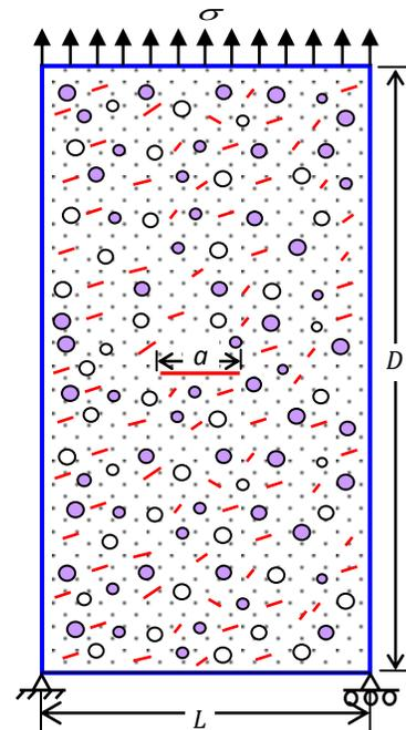
Figure 4. Center crack plate along with multiple holes, inclusions and minor cracks.
