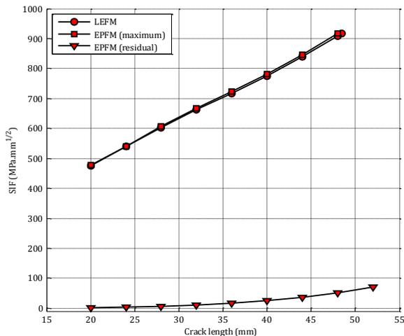
Figure 5. SIF variation with crack length for a center crack plate in the presence of multiple holes, inclusions and minor cracks.
