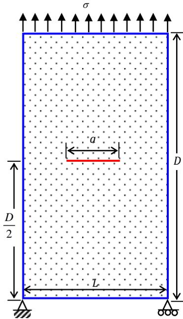
Figure 1. Center crack plate along with dimensions.
