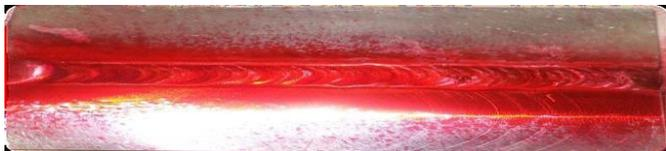
Fig5 Penetrant application on HE15 welded sample
