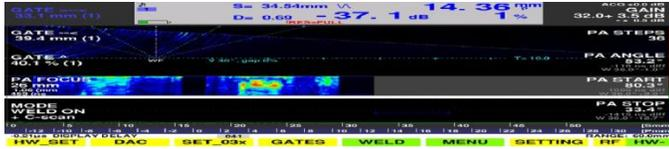
Fig2: Ultrasonic phase array Defectogram of welded HE15 material Defect at 0.69mm depth
