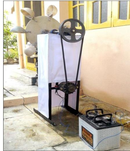
Fig 9: Prototype of the Micro-Hydro Turbine
