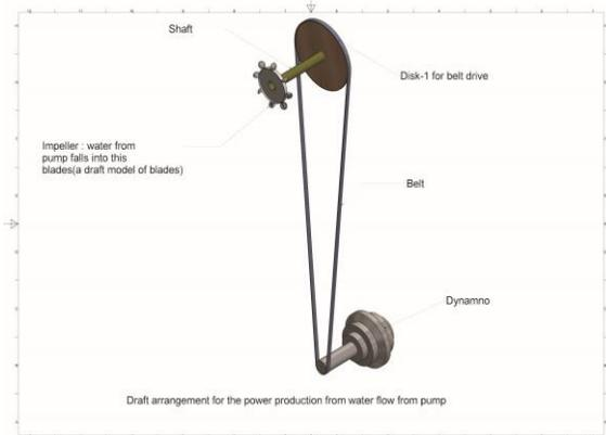
Fig 8: CAD Model of the Micro-Hydro Turbine
