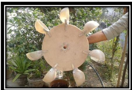
**Fig 4: Fabricated runner with buckets by composite materials**
