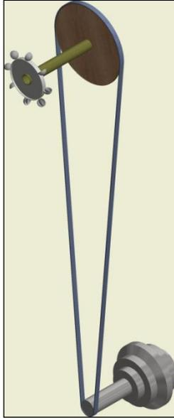
**CAD Model of the Assembly:** In this system we have a wheel arrangement on which the blades are arranged and a shaft is connected to the wheel and the generator (Dynamo) by means of v-belt drive, this dynamo is connected to a battery, in which the power generated by this dynamo is stored and use the power measuring device to measure the generated power.
