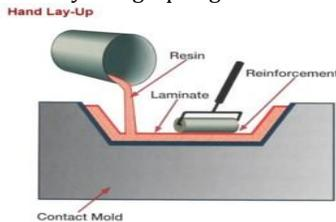
**Fig 3: Hand lay-up method**
