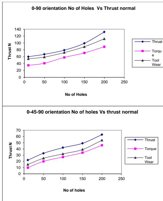
**Fig. 4 Variation of Performance Measures using Normal geometry with respect to Holes**
