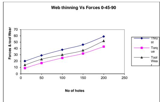
**Fig. 5 Variation of Performance Measures using web thinned geometry with respect to Holes**
