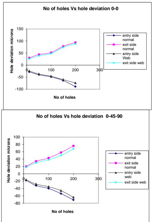
**Fig. 6 Hole deviation with respect to No. of Holes**
