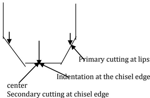
**Fig. 2 Three Components of Thrust Force**
