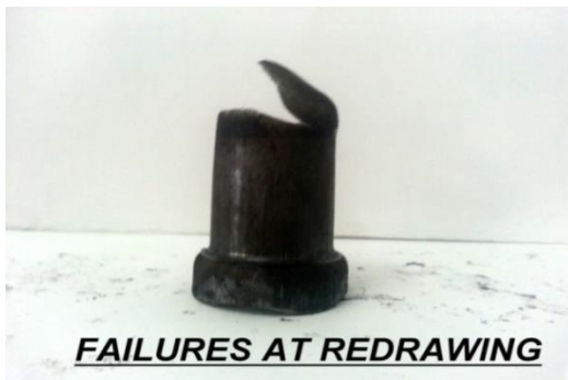
Figure 11 cup failed in redrawing
