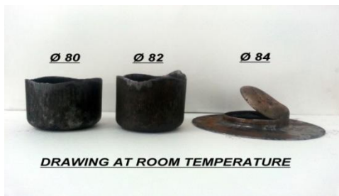
Figure 2 : Various diameter cups drawn at room temperature
