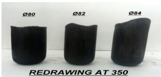
Figure 10 cups redrawn at 350°C
