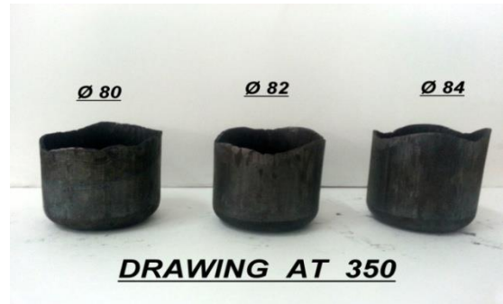
Figure 5 cups of various diameters drawn at 350°C
