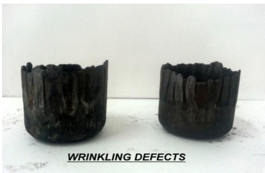
Figure 12 Drawn cups with wrinkling defects
