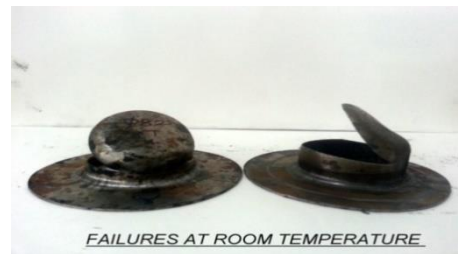
Figure 6 cups failed at room temperature
