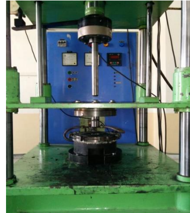
Figure 1 Direct redrawing die assemblies
