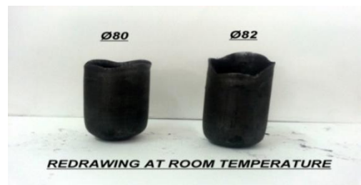
Figure 7 cups redrawn at room temperature
