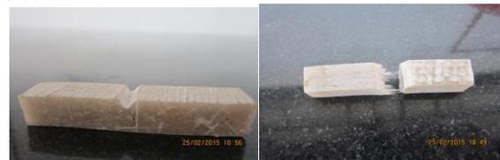
**Fig 7: impact test specimens before and after striking the pendulum**
