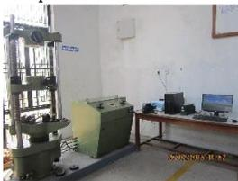
**Fig 3: UTM setup**
