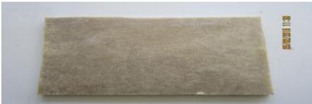
**Fig 2: Hybrid composite laminate**
