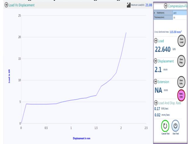
Fig 10: Compressive strength across the fibre orientation
