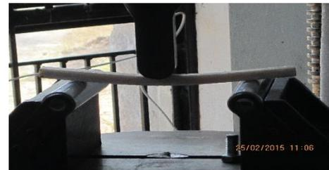
**Fig 6: specimen under flexural test**
