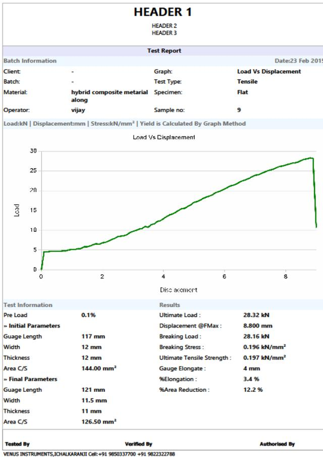
Fig 8: Tensile strength
