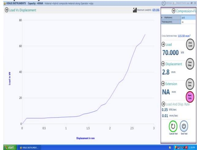
Fig 9: Compressive strength along the fibre orientation
