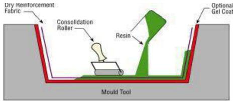
**Fig 1: Hand lay-up method**
