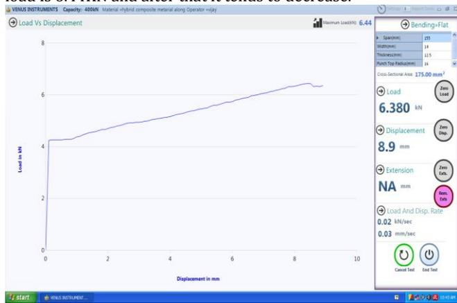
Fig 11: Flexural strength
