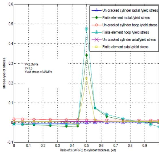
Fig. 7. A cracked cylinder finite element stresses versus an un-cracked cylinder theoretical stresses
