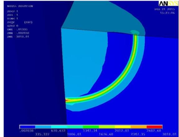
Fig. 5. Stresses at the crack tip
