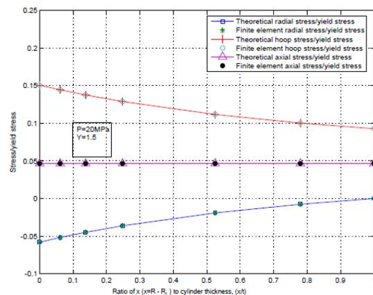
Fig. 6. Theoretical versus finite element stresses
