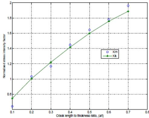
Fig. 10. Comparison of  $K_m$  with  $K_k$  for  $Y=2.0$
