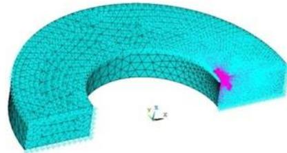
Fig. 2. Refined mesh at the crack tip
