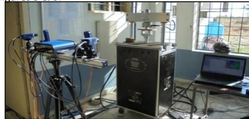
Figure3: Three point bending test with PZT 5 H on the support
