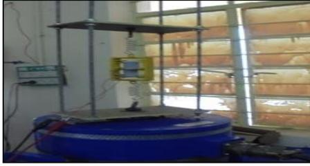
Figure5: Scavenging device on 20 g Syscon Exciter
