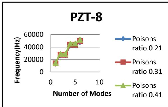
Figure 9: Modal frequencies of PZT-8 disc at different poisons ratios
