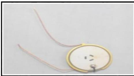
Figure 1: PZT-5H disc with electrodes
