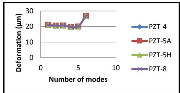
Figure 10: Deformation of different PZTs at 0.31 poisons ratio
