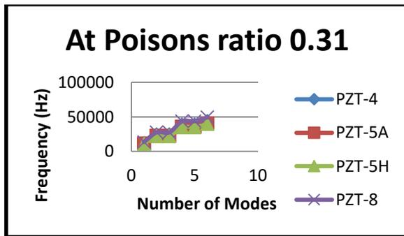
Figure 8 : At poisons ratio 0.31 modal frequencies of different PZTs
