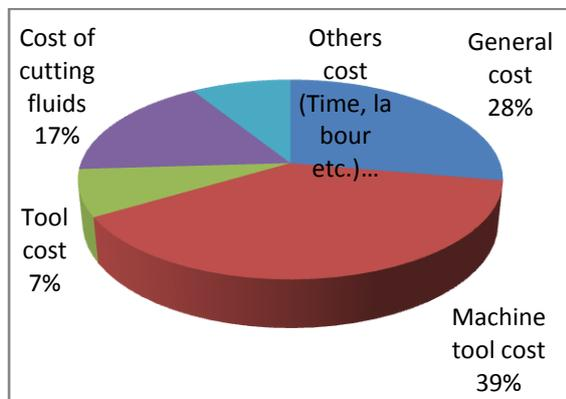
Figure.1 Manufacturing Cost for camshaft Europe by automotive industry
