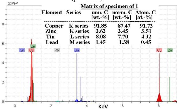
Figure 10: EDS of matrix of sample 1
