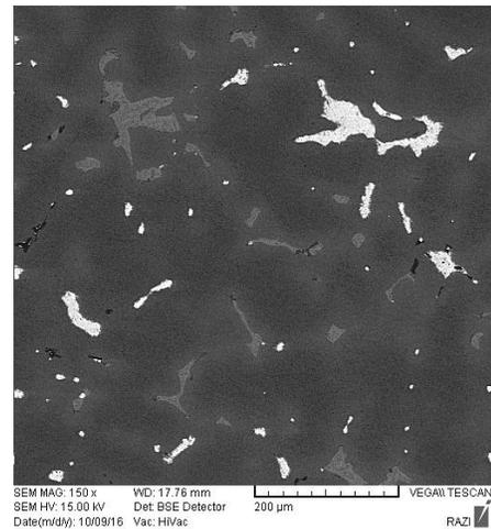
Figure 4: Microstructure of sample 2 at different scales, CuPb10Sn8Zn2 bronze is poured at 950C
