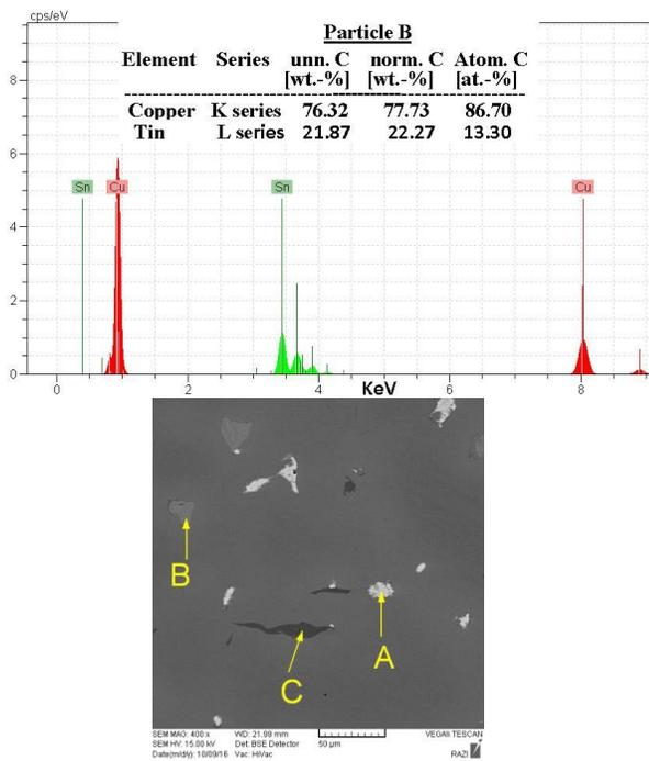
Figure 5: EDS of the solid solution of copper-tin (particle B)
