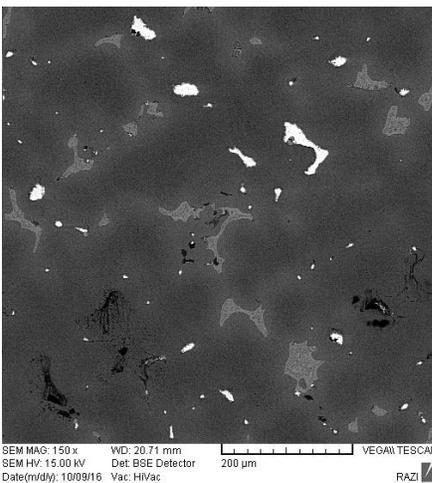
Figure 3: Microstructure of sample 1 at different scales, CuPb10Sn8Zn2 bronze is poured at 1200C
