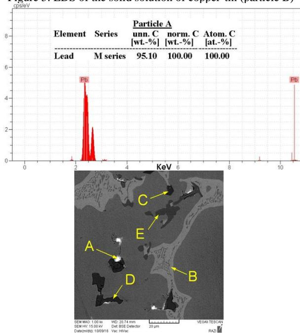
Figure 6: Pure lead phase EDS (Particle A)
