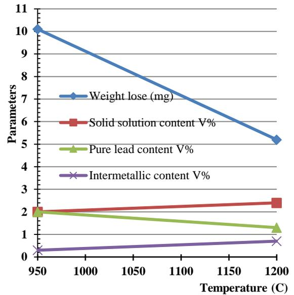
Figure 12: The relationship between the grain size and phase values with weight loss due to wear
