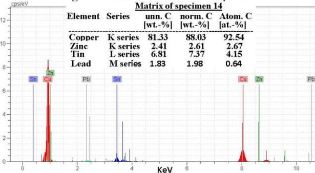
Figure 11: EDS of matrix of sample 2
