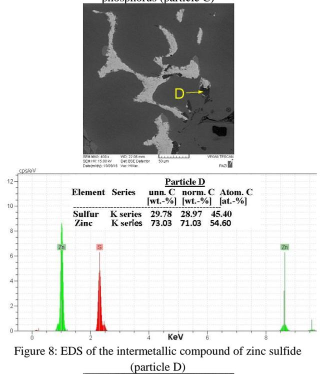
Figure 8: EDS of the intermetallic compound of zinc sulfide (particle D)
