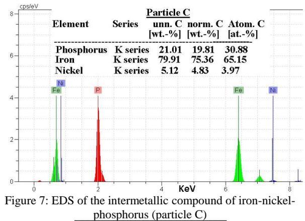
Figure 7: EDS of the intermetallic compound of iron-nickel-phosphorus (particle C)
