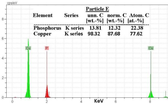
Figure 9: EDS of the intermetallic compound of phosphor-copper (particle E)
