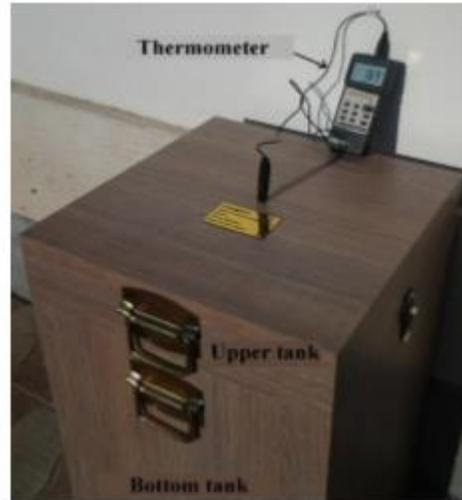
Figure 2: Sub-zero treatment equipment
