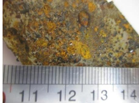
Figure 2: Sample image after 168 hours of corrosion
